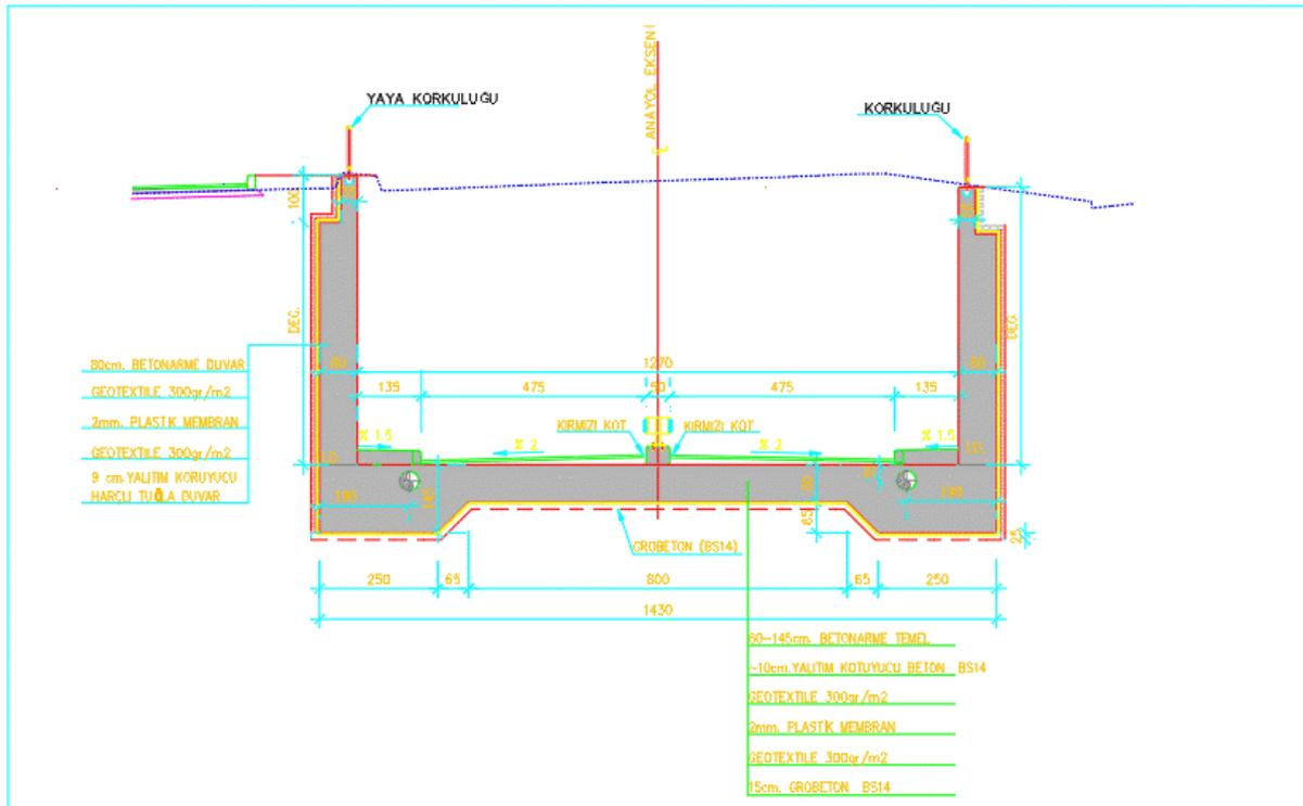
Picture 28 Trabzon Gündoğdu Project concrete U section details
