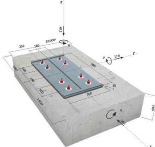
Picture30 Steel Bridge Anchor details computer modeling
