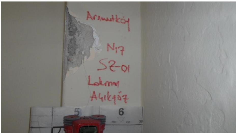
Picture60 Core taking from the building, corrosion control and reinforcement x-ray
